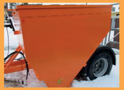
The sand spreader cart is available in three different models with a capacity of 7.5 m<sup>3</sup>, 5 m<sup>3</sup>, or 3 m<sup>3</sup>.
